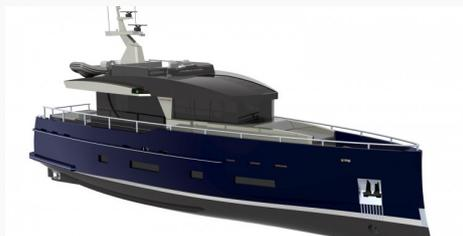
The standard 'displacement' version will have a steel hull and a GRP superstructure. She will be powered by two 250hp engines allowing her a 1,500 nautical miles range at 10 knots. Bering Yachts will also offer an option for Hybrid Propulsion using the ReGen Nautic electric hybrid system. This will reduce the usage of fossil fuel, providing the power needed at sea, and will allow the ability to enter and leave ports in electric-only mode.
