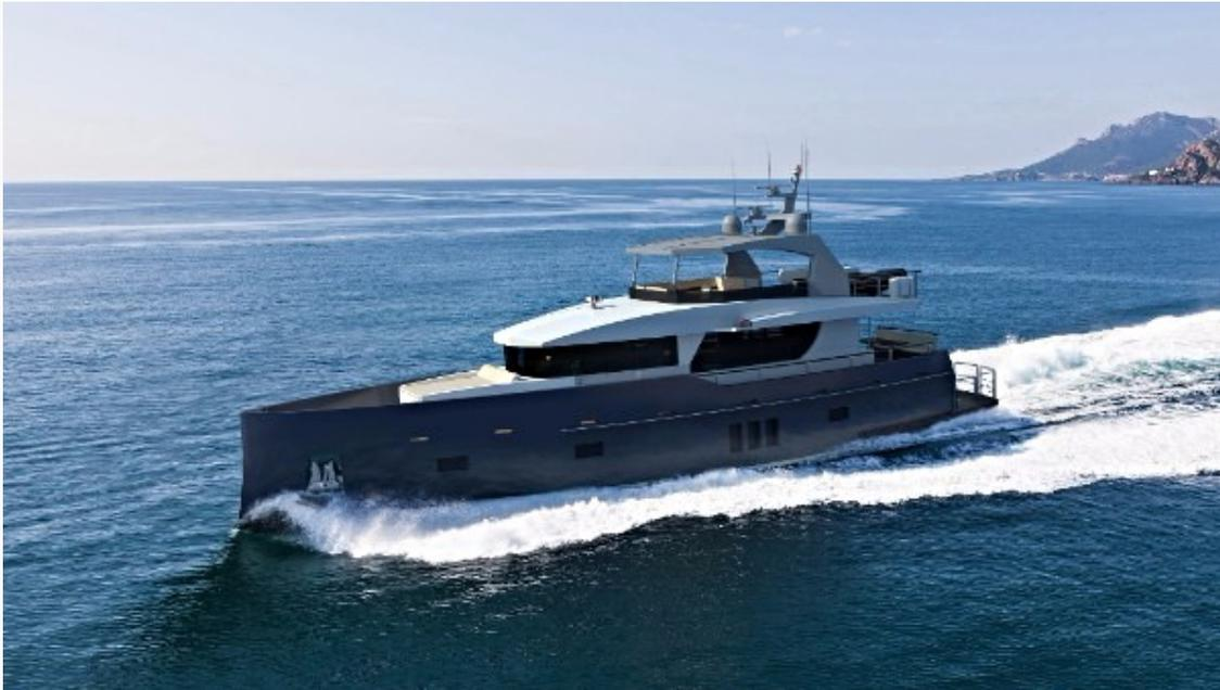
*Designed for wave piercing performance, Bering 85 will be able to cruise for 3,500 nautical miles at 8.5 knots burning a combined 8.5 gallons per hour.*
