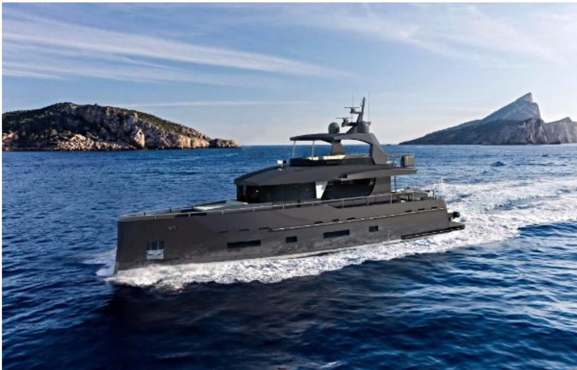
*Bering 70 Tempest will be completely made out of aluminum and will be able to reach a top speed of 22 knots*
